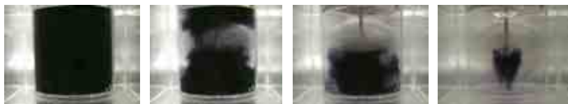
Fig.1 N=3s^{-1} , Re=20 ( \rho=1,350kg/m^3 , \mu=1.0Pa\cdot s ), D=0.124m , H=0.083m , d=0.07m , b=0.014m
