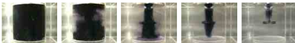
Fig.2 N=3s^{-1} , Re=15,000 ( \rho=1,000kg/m^3 , \mu=0.001Pa\cdot s ), D=H=0.17m , d=0.07m , b=0.014m
