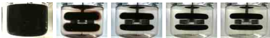
Fig.1 N=3s^{-1} , Re=20 ( \rho=1,350kg/m^3 , \mu=1.0Pa\cdot s ), D=0.124m , H=0.083m , d=0.07m , b=0.014m
